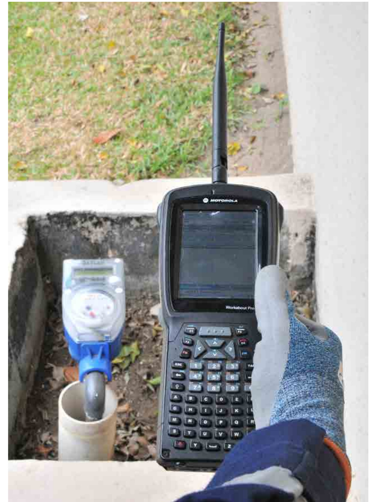
SODECI water meter readings with MDAT (Mobile Data Acquisition Terminal)
